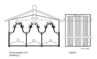
Figure 1. Cross-section and layout of the poultry confinement buildings.
